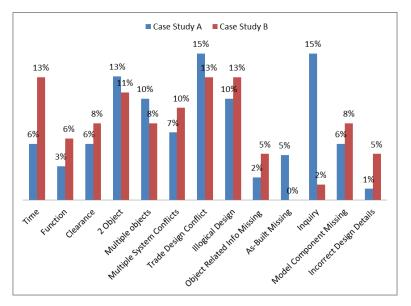
Figure 9: Analysed BIM design coordination issues in case study A & B (% of total issues analysed)
